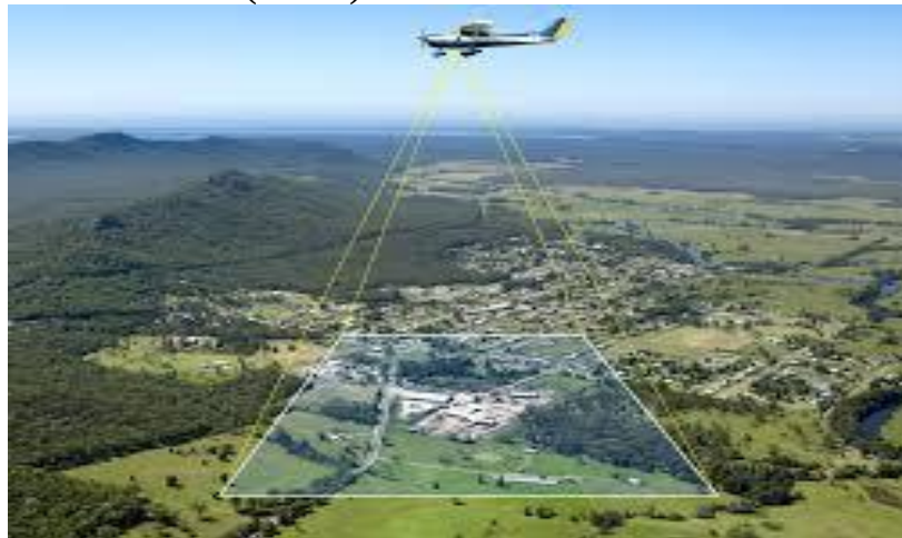
Fig: Aerial Photogrammetry
